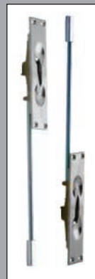
Top and Bottom Manual Flush-Bolts Applied to the leaf opposite the leaf with the lock-set. Standard ANSI 6 3/4" x 1". Finish to match the door and frame finish.
